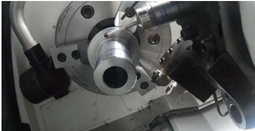
This photo shows measurements taken along the Y-axis by an LB3000 EX III with Y-axis specs.
