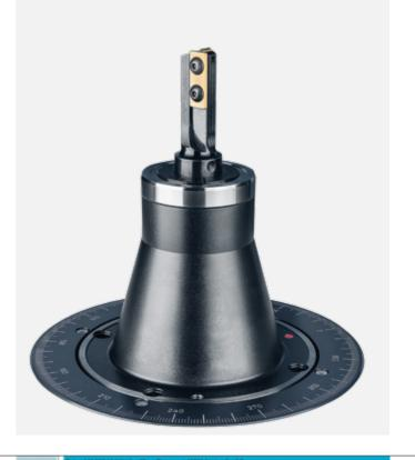
**2 | The automatic measuring procedure** delivers results for the tool in one or two planes. After the measurement, click to rotate the tool to the right position and correct the imbalance.
