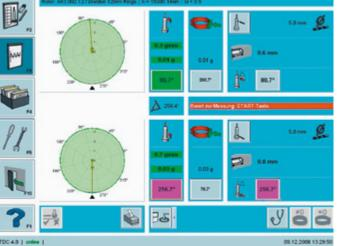
3 | A laser marking displays the balancing point to identify the imbalance so it can be corrected. After the imbalance has been corrected by adding or removing mass, another measurement can be completed. The result and quality grade can be output as a protocol.
