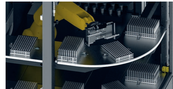
Only with »roboSet 2«: 8 pallets on 2 levels
